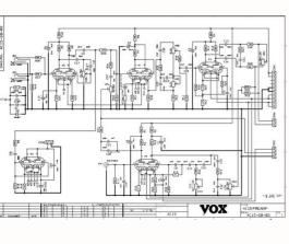
Vox ac15 handwired schematic. Vox ac15 top boost schematic. Vox ac15 heritage handwired schematic. Vox ac15 schematic layout. Vox ac15 clone schematic. Vintage vox ac15 schematic. Vox ac15 schematic pdf. Vox ac15c1 schematic.
